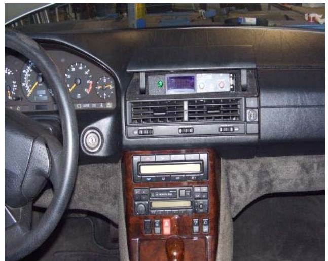
Vari-Cool Methanol Controller, Wide-Band Aor/Fuel Display & Methanol Flow/Pressure L.E.D. light installed into hidden dash compartment
