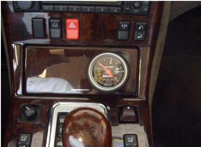
Boost Gauge with Memory High Boost recall and Overboost Warning. Installed with Angle cup to direct the gauge towards the driver.
