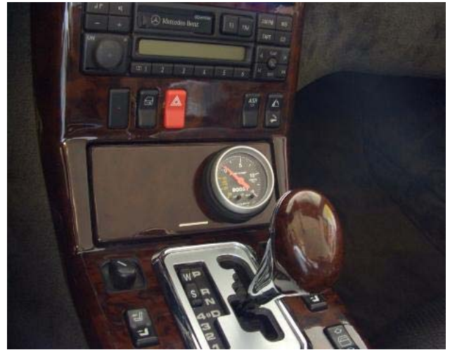
Boost Gauge with Memory High Boost recall and Overboost Warning. Installed with Angle cup to direct the gauge towards the driver.
