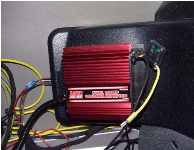
MSD Fuel Pump Booster Increases voltage to the fuel pump during boost conditions.
