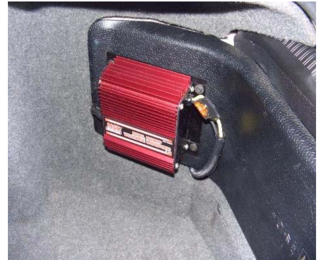
MSD Fuel Pump Booster Increases voltage to the fuel pump during boost conditions.
