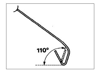
1.4 In the marked area (A), the fender flange is flattened down up to the inside of the fender in several stages. A plastic hammer must be used to avoid damaging the paint.
