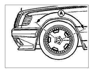
1.5 Allow front fender flare to curve smoothy back towards original, unflared line within the marked area (B).
