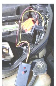
Pictured here is the code reader connected to the diagnostic module of a 94 E320 (w124). The red wire is plugged into pin 16 and the black wire is plugged into pin 1. The yellow/white wire is plugged into the other pins (as described by the code description files) to read codes for a specific system.
