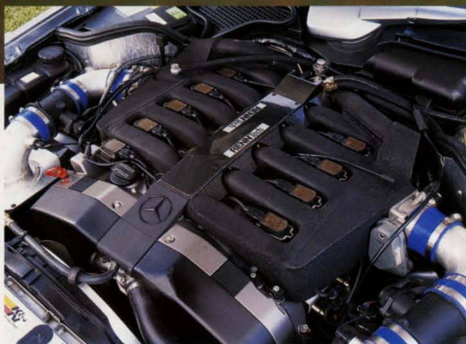
Our long-term E320 (above) was in for an extensive makeover, especially in the engine compartment, where RENNTech shoehorned in a potent 7.4-liter V-12 (right).
