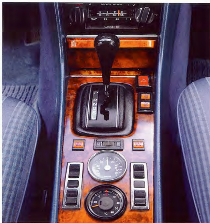
The ammeter, exterior temperature display and switches for the belt "de"-tensioning system (top right) identify the 6.9 as a prototype model
