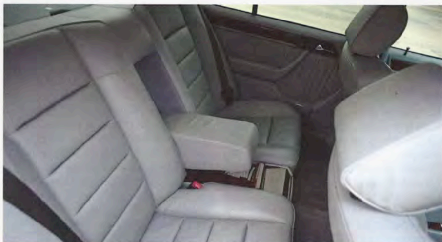
Unique to the 500E was a four-place passenger cabin that used Recaro Sportline bucket seats front and rear, giving the car another unique characteristic among W124 E-class machines.
