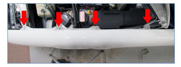
• Remove these 4 bolts last and lift the fender off of the car.
