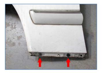
Two more bolts are revealed at the front of the fender once the bumper is off.
