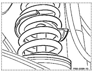
1.6 Unscrew upper fixing nuts (75a, 75e) of piston rod (60).
