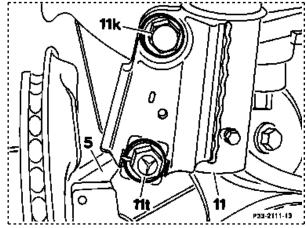
1.13 Secure steering knuckle using suitable bracket.
