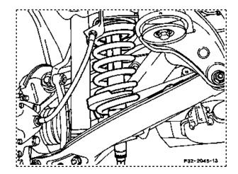
2.3 Fit upper rubber ring to shock absorber, install in spring link and assemble lower screw
