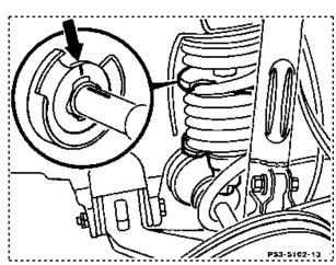
If there is inadequate assembly clearance, unbolt left axle shaft (inner) at axle shaft flange.
