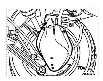
1.3 Install clamp 000 589 46 31 00 and clamp spring until spring link is relieved of load.
