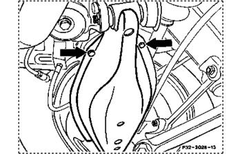
1.4 Install clamp 000 589 46 31 00 and clamp spring until spring link is relieved of load. The spring clamp should engage at least 5½ spring coils.
