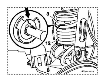
1.6 Unscrew nuts from eccentric bolts. Press out eccentric bolts on front and rear control arm mounting and lower control arm.
