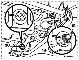
2.5 Secure damper piston rod in upper damper
