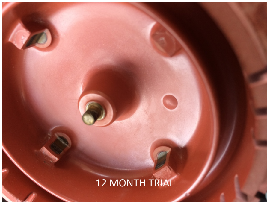
Figure 43 Modified Distributor Cap - Type 2 - At 12 months During Road Test - 3000 Miles
