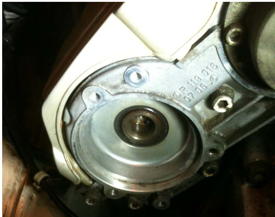
Figure 51 Photo of Alloy Recess (No Corrosion)
