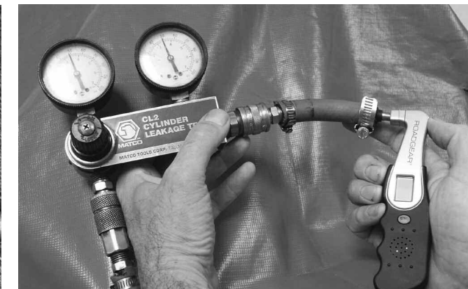
Each gauge was tested twice at three pressures; 20, 35 and 50 psi and the MATCO was zeroed and recalibrated between each reading. After this testing, we conducted durability testing after two 40" drops to a concrete floor.
