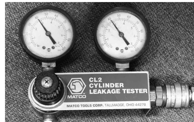
Testing was done using a MATCO leak down tester calibrated with a racing-type $395 Intercomp digital gauge guaranteed accurate to .5%. This leakage tester also has a very fine pressure regulator.
