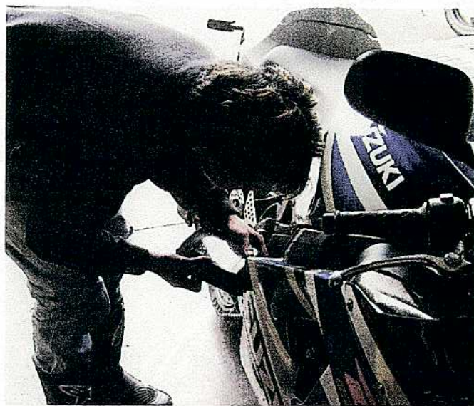
We ran both bikes with standard petroleum automobile oil (Valvoline 10W-40) to do our baseline dyno runs. We then drained the oil, changed oil filters and ran the synthetic oil for at least 15 minutes to circulate it through the engine.
