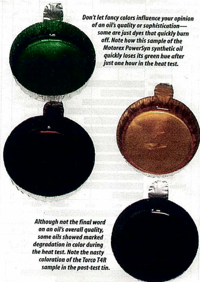
This photo of two oil samples before and after the heat test shows how some of the Group III synthetics are now using better-quality base stocks. The two top tins show Castrol Syntec automobile (left) and Motul 300V (right) before the heat test; the two lower tins are both oils afterward (again, Castrol left, Motul right). Note the similarity in color between the oils in the post-heat test samples.
