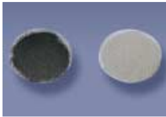
Soot quantity in the filter paper three minutes after the cold start. Afterglow (right) cuts the soot quantity by approx. 40 %.
