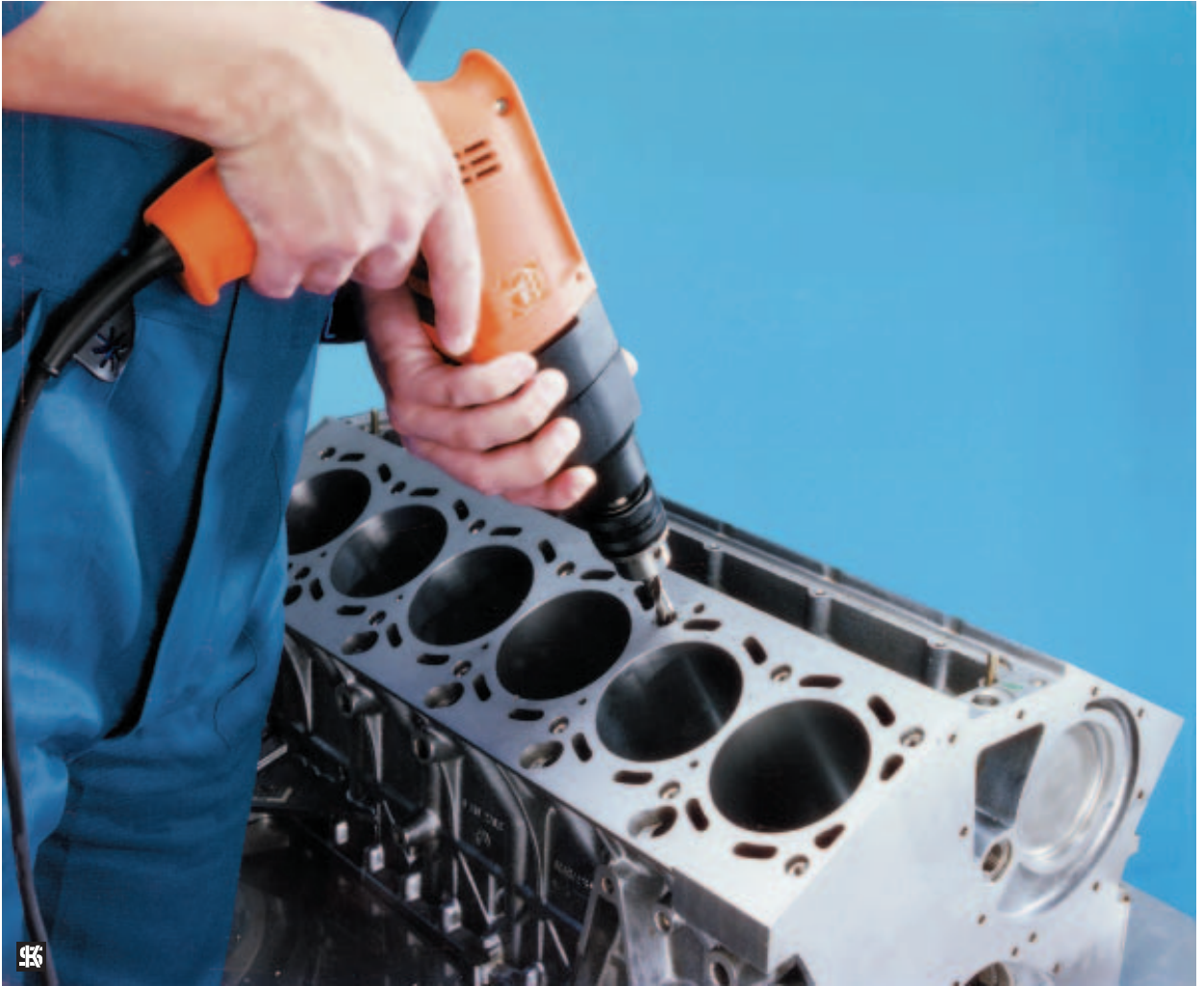
Figure 13 Drill a core hole with a drill or bore the old thread out
