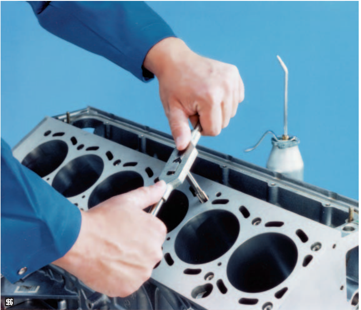
Figure 15 Cutting the thread with a tap
