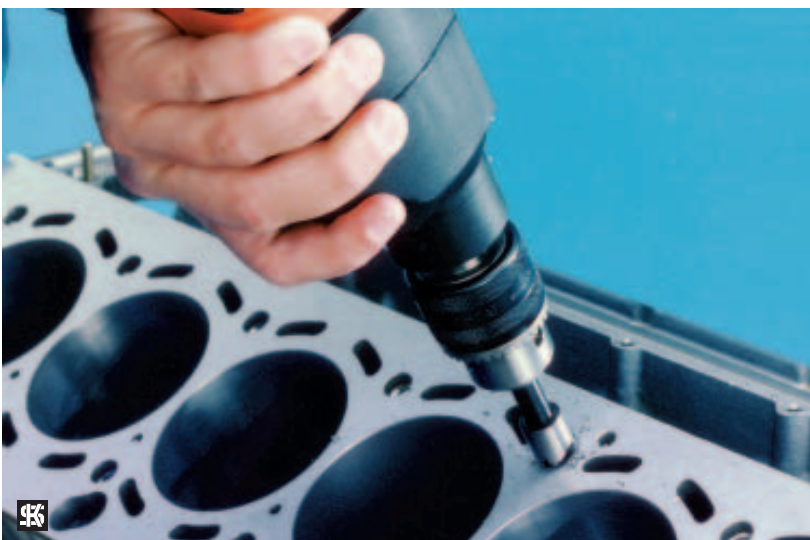
Figure 14 The core hole is countersunk with a shank cutter (depth 2.5 mm).
