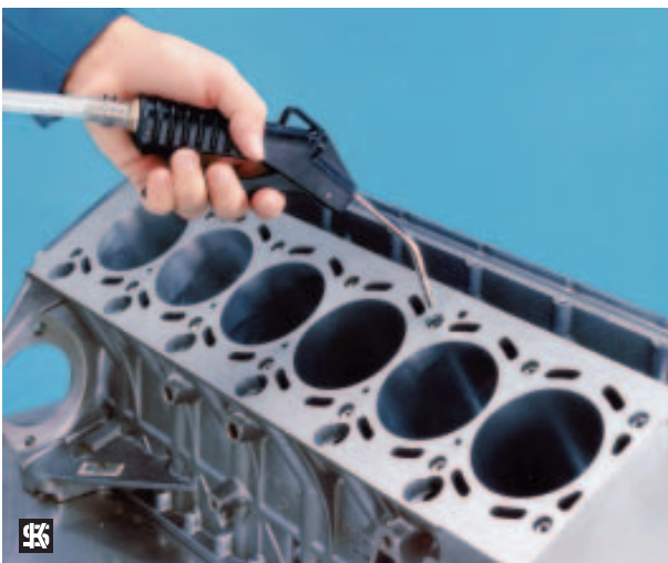
Figure 16 Important: Blow out chips and oil
