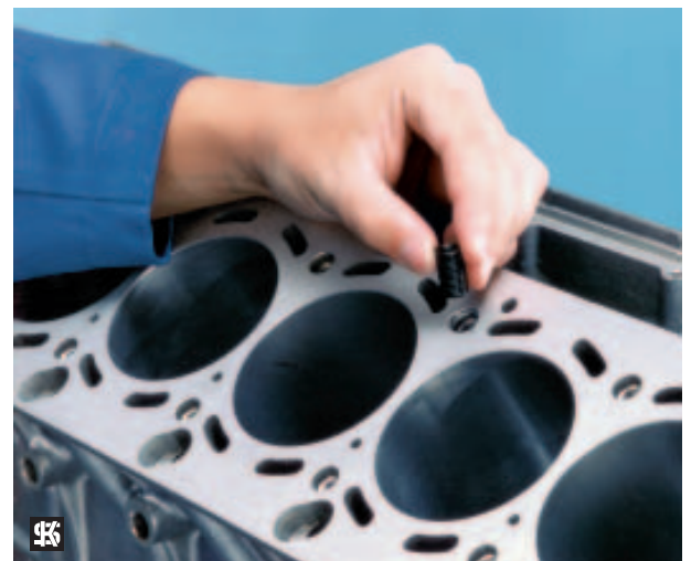
Figure 17 Position threaded bush by hand and screw a few turns
