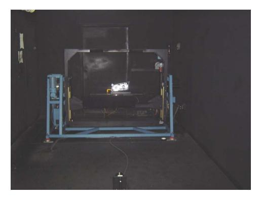
Figure 8. Photometric laboratory instrumentation with a headlamp mounted on the goniometer table. The photometric sensor is located 100 feet from the center of the headlamp's bulb filament at the opposite end of the tunnel.
