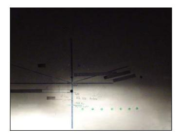
Figure 12. A TYC Ford Taurus low beam when aimed using the VOR method.
