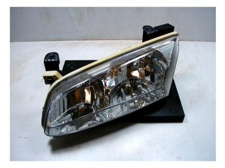
Figure 7. 2000-2001 LH Toyota Camry headlamp mounted on the photometric test fixture.
