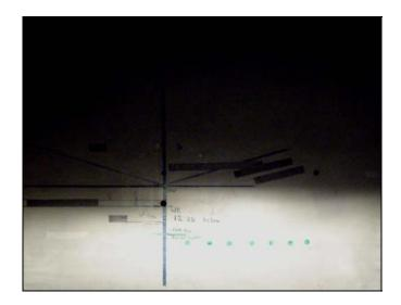
Figure 13. An original equipment manufacturer (OEM) replacement Toyota Camry low beam pattern aimed using the VOR method.
