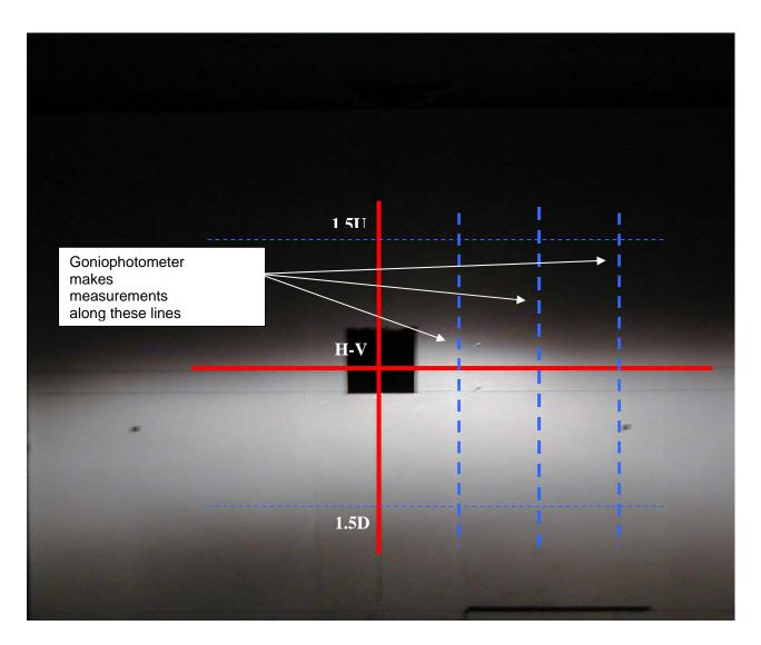
Figure 1. Representation of the VOR aiming grid laid over a headlamp beam pattern. Proper vertical aim of the headlamp is carried out by the goniophotometer.
