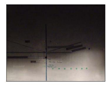
Figure 14. A TYC Toyota Camry low beam pattern aimed using the VOR method.
