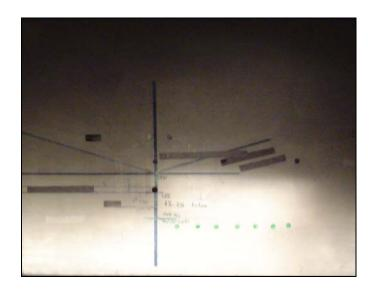
Figure 15. A DEPO Toyota Camry low beam pattern aimed using the VOR method.
