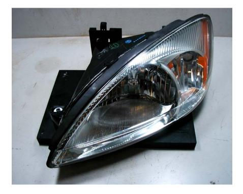
Figure 5. 2000-2003 LH Ford Taurus headlamp mounted on the photometric test fixture.
