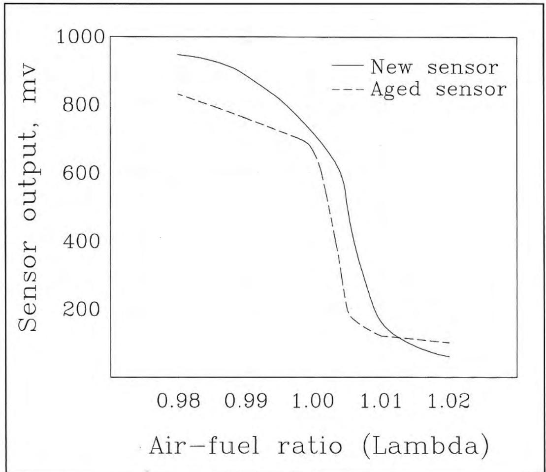
Most folks don't have a CO meter, but many have a multi-meter. It is tempting to gauge exhaust CO on the basis of the output of a lambda (oxygen) sensor, but beware that the sensor's output sags gradually with age, so simply aiming for about 500 millivolts may not do the trick. The shape of the curve is reliable, however, so by adjusting the mixture both rich and lean, you can establish the upper and lower limits of the sensor's output range. Aim for the middle.
