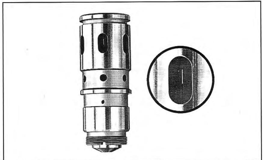
The position of the control plunger relative to the extremely narrow (about 0.008 in) slits in the metering barrel controls the rate of fuel flow in the K-Jetronic system. (Robert Bosch Corporation)
