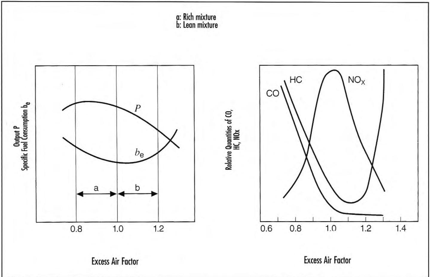
Burning fuel with insufficient air results in carbon monoxide (CO) being formed, instead of carbon dioxide (CO<sub>2</sub>). Excess fuel also leaves unburned hydrocarbons (HC) in the exhaust. Paradoxically, a too-lean mixture causes misfires, which also lets unburned fuel escape. Oxides of nitrogen (NOx) are produced in greatest abundance when the mixture strength is just a bit lean, when combustion is hottest. (Robert Bosch Corporation)
