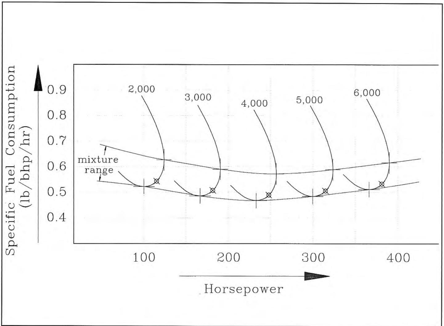
A series of fish hooks established at various engine speeds produce, when linked together, a curved band that represents the practical range of mixture strengths for any given engine. The line forming the upper boundary of this band represents the mixture curve for maximum power; the lower one for maximum economy.
