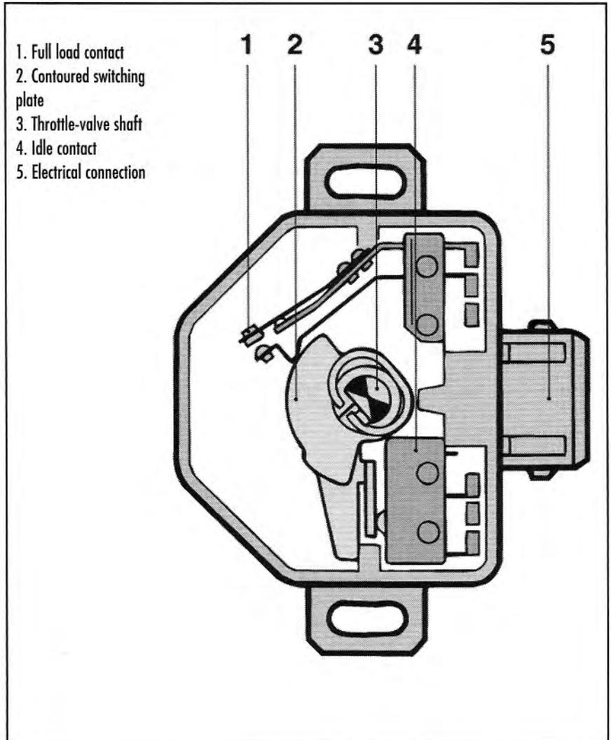
**At idle and at full-throttle, lambda controlled systems ignore the sensor and revert to "open-loop" operation, using their preprogrammed maps to decide the length of injection pulses. The change between modes is signalled by the throttle switch. (Robert Bosch Corporation)**
