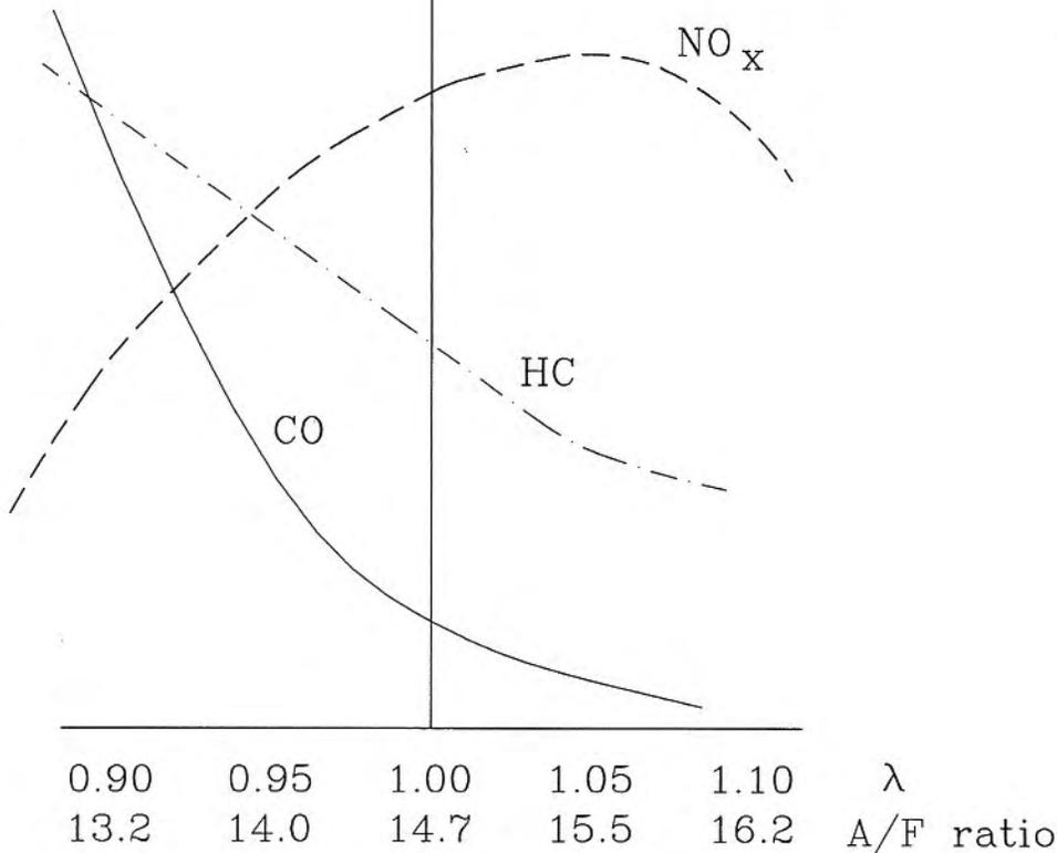
Three-way catalytic converters are essential to meet current emissions limits. But converters can only do their job if the air/fuel mixture fed to the engine is held very close to stoichiometry—the chemically correct ratio. And to achieve that, a lambda (oxygen) sensor is essential. Its electrical output varies very strongly right around the point of stoichiometry.
