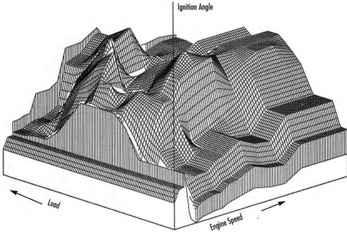
**Motronic ignition advance (top) compared with map of a conventional mechanical system (bottom). Electronic control over ignition timing, based on numerous inputs, permits finer and much more detailed control over spark advance, maximizing performance without risking detonation. (Robert Bosch Corporation).**
