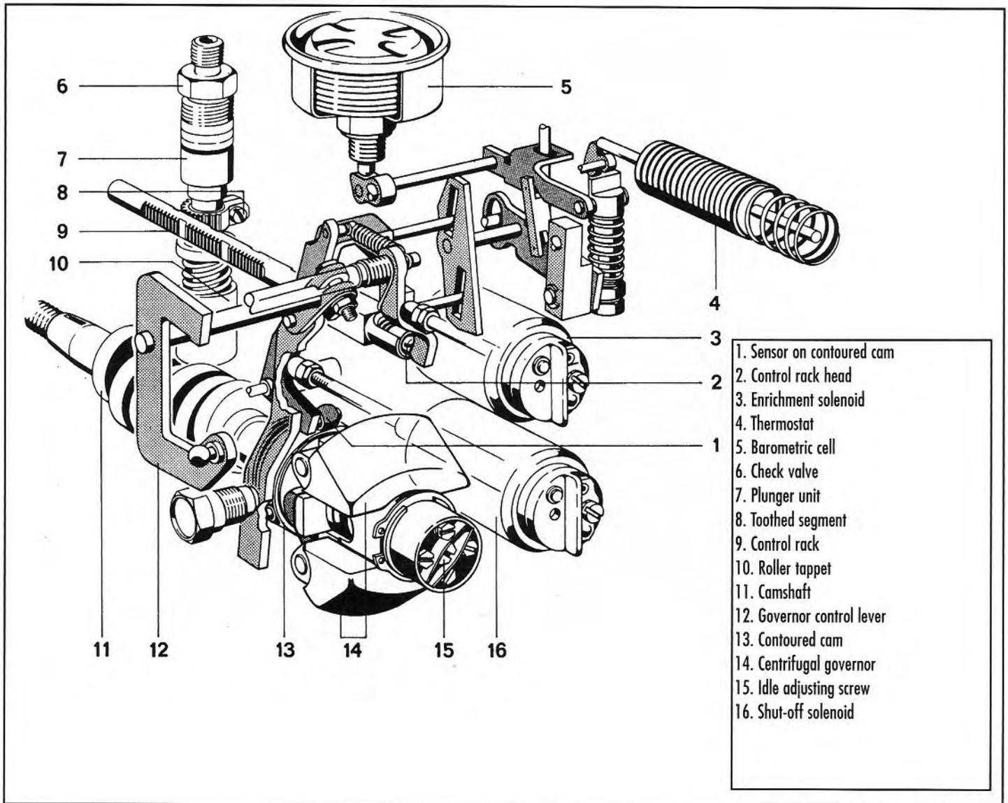
The complexity of the mechanical controls for the Bosch system used on the 300SL is mind-boggling. Fuel delivery of the pump (only the camshaft is shown, 11) is controlled by the rack (9). The position of the rack is governed by engine speed, via the centrifugal weights (14) acting on a contoured cam (13), and by throttle position. Other factors are accounted for by a barometric capsule (5) and a temperature sensitive device (4). (Robert Bosch Corporation)
