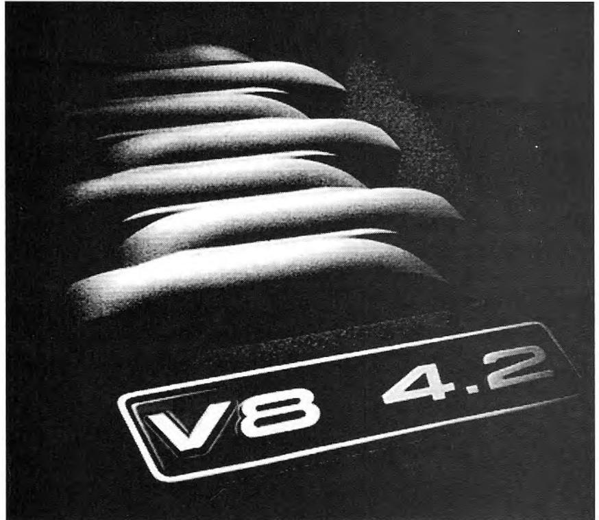
Tuned-length intake pipes can provide a degree of "acoustic ramming," pumping up the torque curve at an rpm that depends on the length of the pipes. Long ones, as on this Audi twin cam V8, beef up the bottom end of the range; short ones add top end power at the expense of low end torque. (VW Canada)
