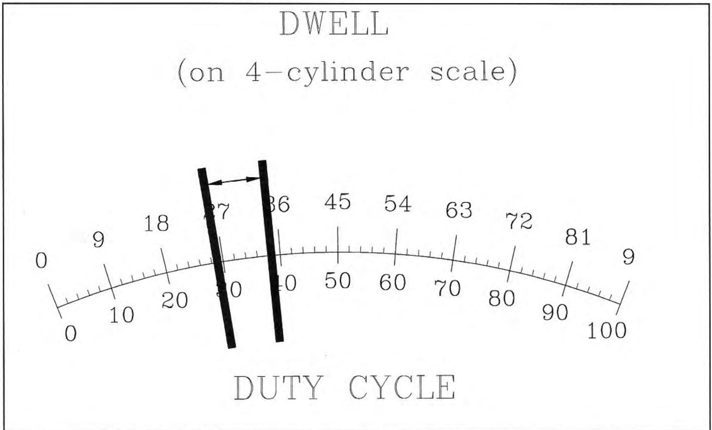
A reading around 25–35 degrees (about 30–40% duty cycle) means the lambda valve is trying to raise the control pressure to lean out an excessively rich mixture.
