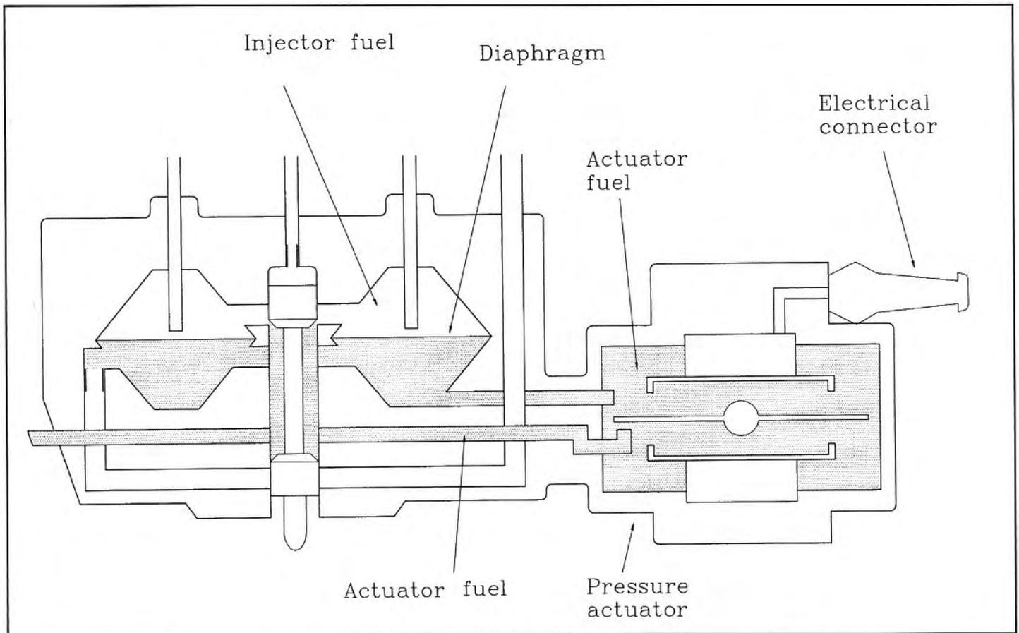
**KE systems impose a fixed resistance to flow out of the lower chambers of the differential pressure valves and vary the pressure going in by having a powerful electromagnet bend a thin steel plate toward or away from the supply port.**
