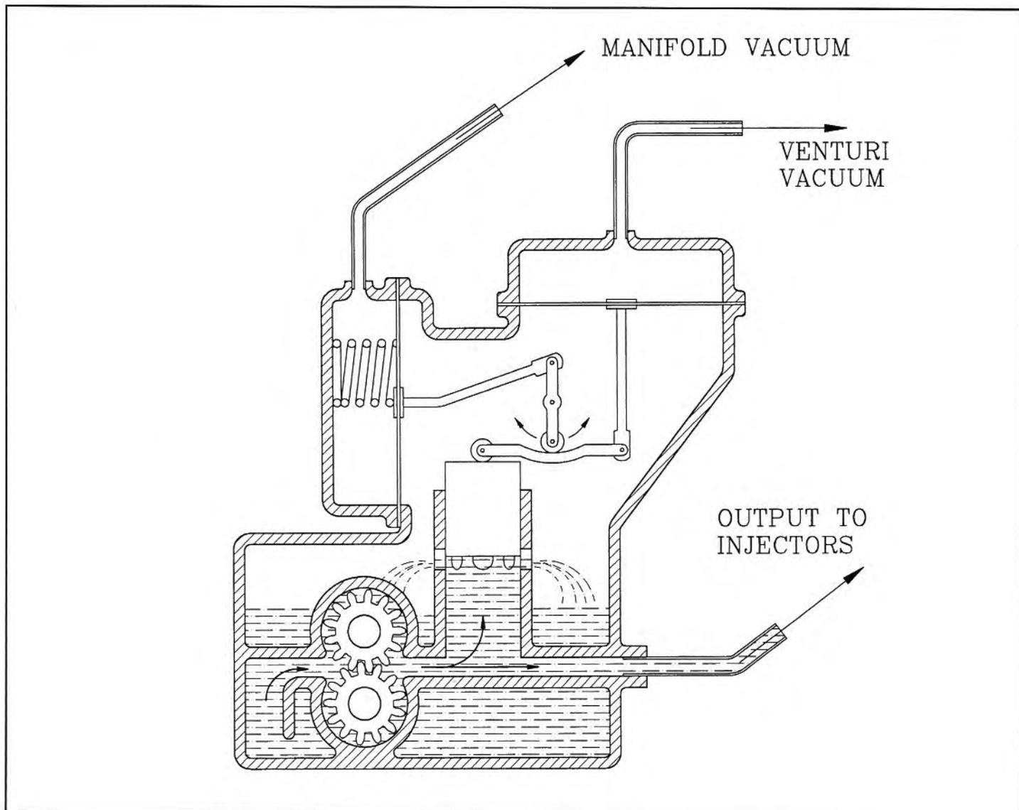
The heart of the Rochester system's control unit was a spill valve that returned to the tank a certain fraction of the fuel delivered by the gear-type pump. The position of the piston in the spill valve was determined by two diaphragms—one hooked to a manifold vacuum, one to a single large metering venturi that fed the air box. A system of links and rollers linked movement of the diaphragms to the spill valve piston.
