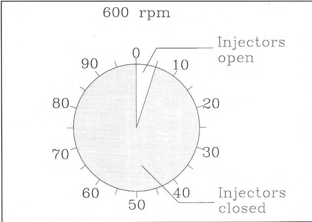
Intermittent Injection systems vary the amount of fuel delivered solely by varying the "on-time" to "off-time" of the electromagnetic injector. At idle, the injectors may only be "on" five percent of the time; at medium revs and load, they may spend more than half the time "on."
