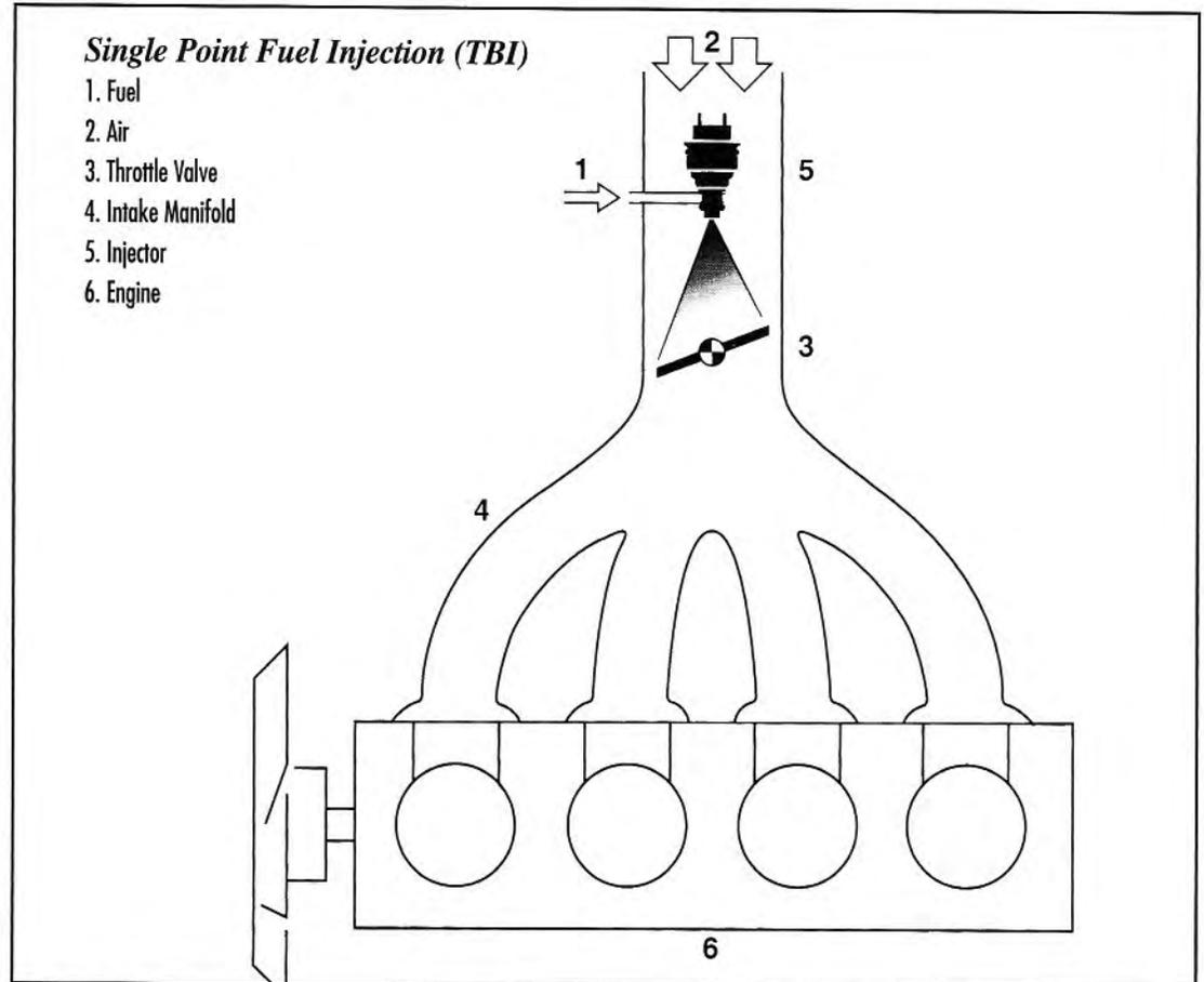
**Introducing fuel at a single point—whether from a carburetor or a throttle body injector—"wets" a large area of manifold surface, and gives unevaporated droplets many chances to drop out, forming puddles of fuel. (Robert Bosch Corporation)**
