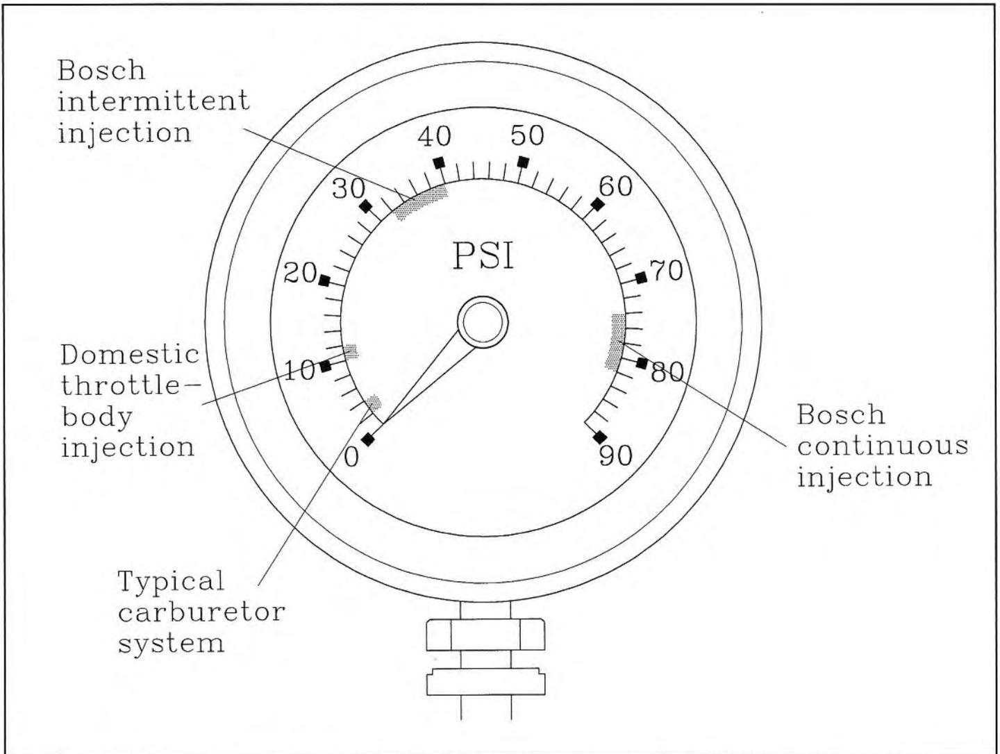
One of the minor reasons why fuel injection is superior to carburetors is because forcing the fuel through small orifices at high pressure does a better job of vaporizing it than sucking it through small orifices with a small pressure difference. A potential downside for servicing is an increased fire risk. Many circuits contain fuel under residual pressure, even when the engine is stopped.
