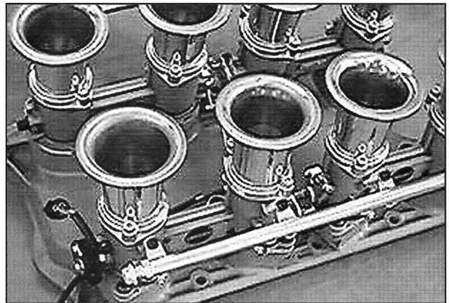
**A British firm, Jenvey Dynamics, offers throttle bodies in both side-draft and down-draft configurations. These are suitable for use with do-it-yourself EFI systems using Bosch fuel-handling and electrical components, and an aftermarket ECU, such as Haltech's. (Jenvey Dynamics Ltd)**
