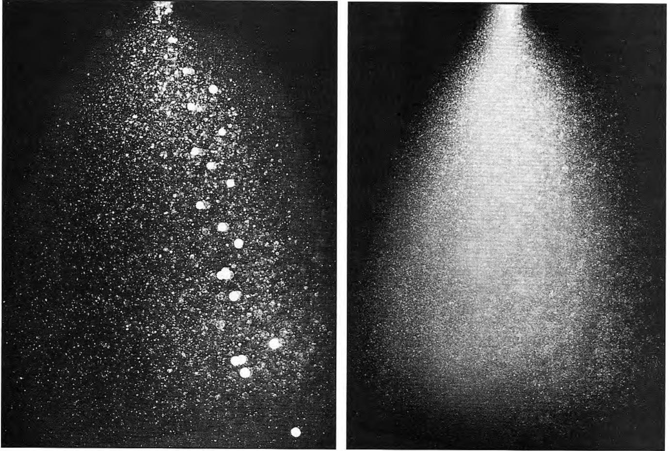
Air-shrouded injectors (right) allow a little of the engine's intake air to pass through the injectors themselves, mixing with the fuel as it does so. Very much like the emulsion tube(s) in a carburetor, this improves atomization. (Robert Bosch Corporation)
