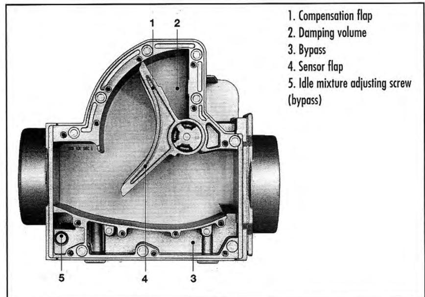
**The vane-type air meter of an L-Jetronic system, viewed from the other side. Note the compensating flap which serves both as a counterweight and as a pulsation damper. (Robert Bosch Corporation)**
