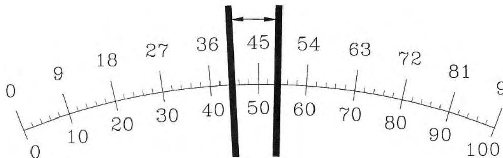
An ordinary dwell meter, set on the four-cylinder scale, can read the duty cycle of the lambda valve. If the basic mixture strength is correct, the meter will oscillate around the 45 degree (= 50% duty cycle) point.
