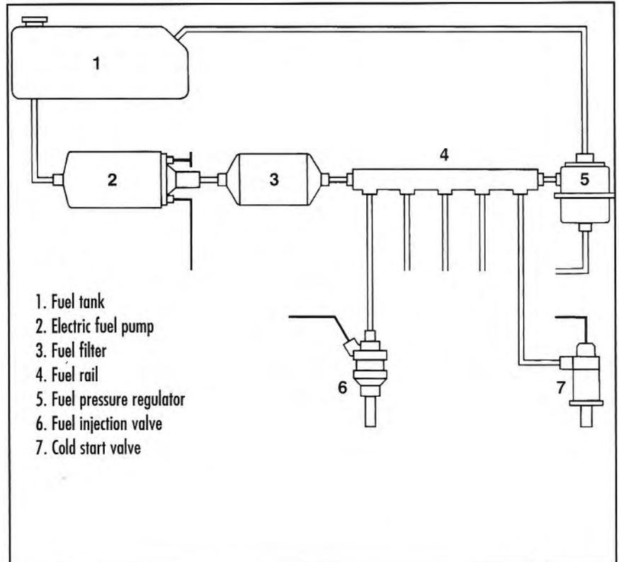
Schematic layout of the fuel supply components of a typical Bosch intermittent injection system. (Robert Bosch Corporation)
