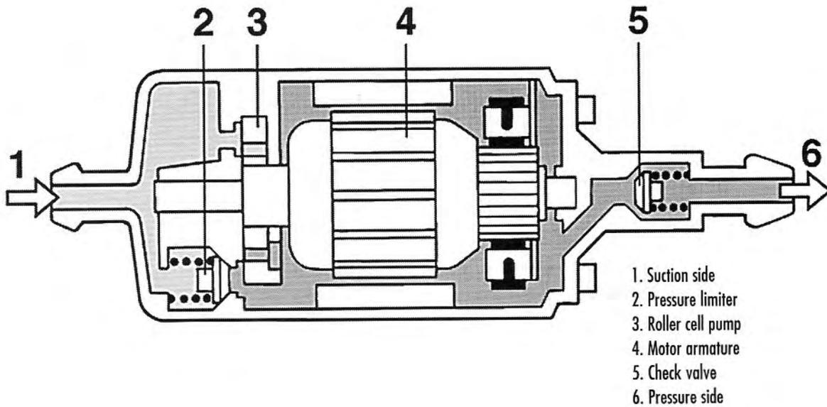
The roller cell fuel pump. The rollers fit loosely in their lands; centrifugal force pushes them against the contoured interior of the pump body. (Robert Bosch Corporation)
