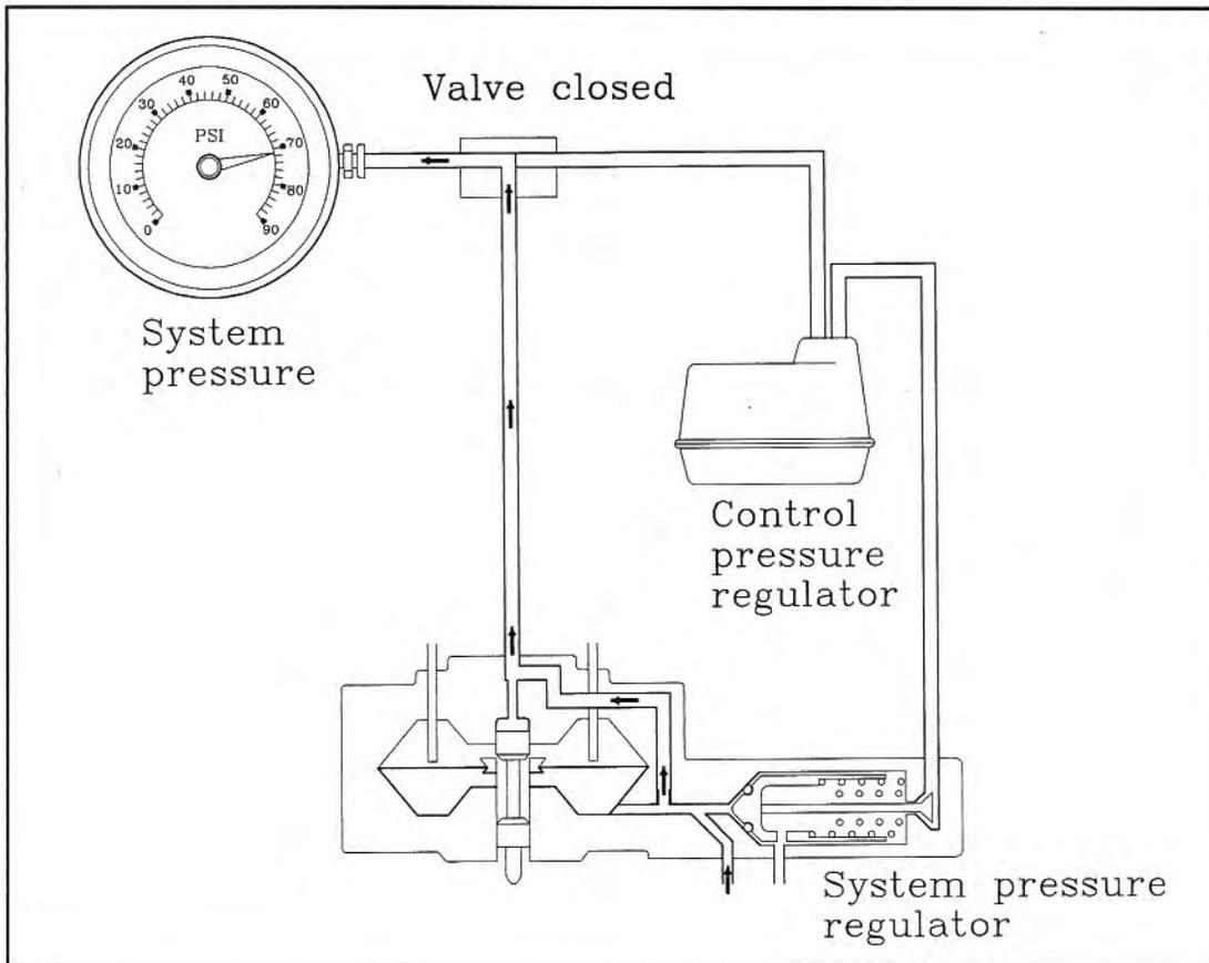
A single test setup permits measuring main system pressure (with valve closed), control pressure (with valve open, see next page), and residual pressure, by using a "Tee" fitting and a shut-off valve (see text). Be sure to use a gauge with a high enough pressure capacity—at least 90 psi.
