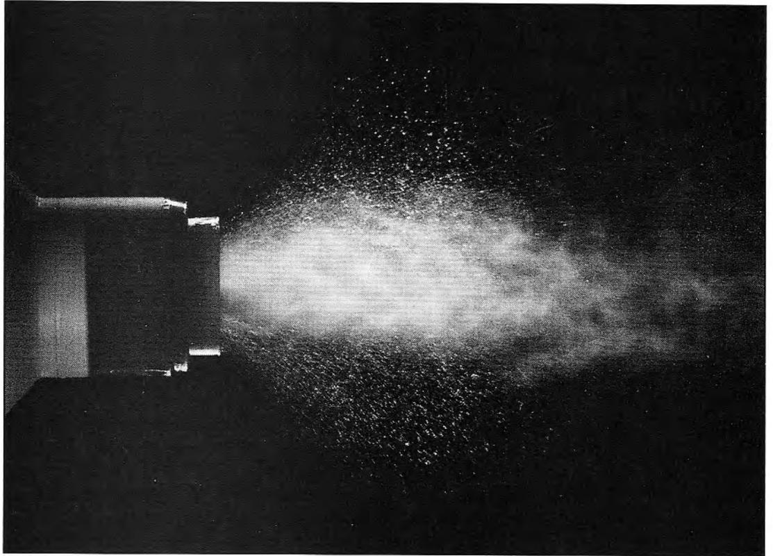
**Ideally, all fuel ingested by the engine would be in the form of vapor. In practice, some droplets remain. Squirting the fuel through a small orifice under considerable pressure improves atomization, which is one reason why fuel injection is superior to carburetors. (Robert Bosch Corporation).**
