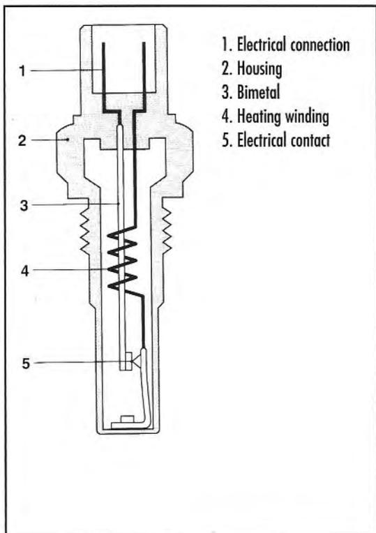
The thermo-time switch. The contacts are closed when the switch is cold, and open when it is hot, either from a warm engine or because the electric heating element has had time to warm it. (Robert Bosch Corporation)
