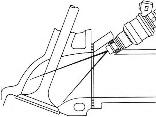
**Multi-point injection also provides the opportunity to locate each injector very near the valve it serves. This reduces port "wetting," and so reduces the amount of enrichment needed for acceleration. (Robert Bosch Corporation)**
