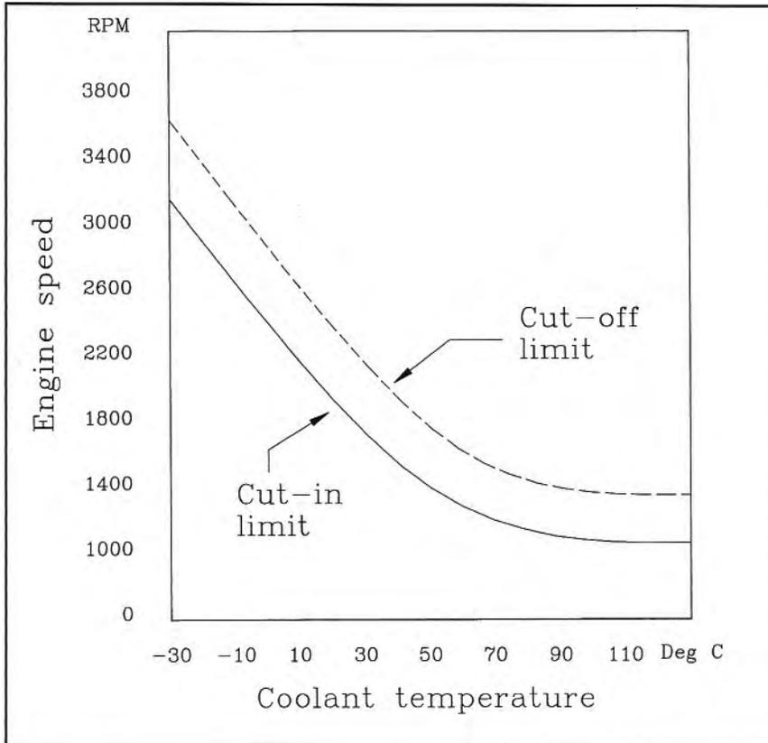
To improve economy and reduce emissions, the fuel is shut off when the throttle is closed, as signalled by the throttle switch. To prevent "hunting," the cut-off and cut-in limits are separated by a few hundred rpm. The rpm at which cut-off occurs is lowered proportionally as the engine warms up, to prevent stalling with a cold engine. (Robert Bosch Corporation)
