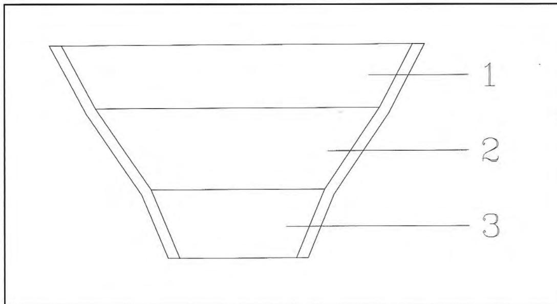
A funnel with multiple tapers allows a comparatively large amount of sensor plate lift around idle, which provides a slight idle enrichment, and a similar richening effect at maximum flow rate, yet with a taper in between the two that gives more rapid vane lift for a given airflow increase—and so a slight leaning—under light load, medium speed operation.
