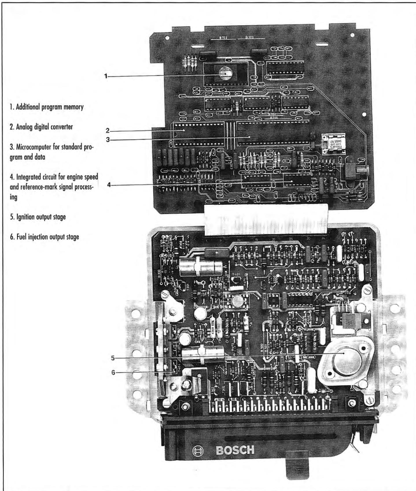
Because the ideal ignition advance depends on mixture strength, and vice versa, optimum results can only be achieved with integrated control over both ignition timing and fuel injection. This is what the inside of the "black-box" that does it looks like. (Robert Bosch Corporation)
