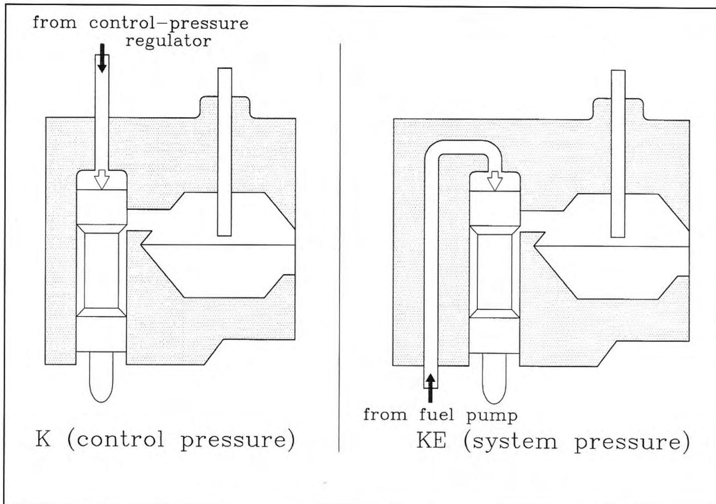
The basic K-Jetronic adjusts mixture strength by varying the control pressure acting on the top of the control plunger, while keeping the pressure drop across the barrel slits constant. In contrast, the KE-Jetronic achieves control over air/fuel mixtures entirely by changes in the pressure drop across the barrel slits; the control force is full primary system pressure, maintained by the primary pressure regulator.
