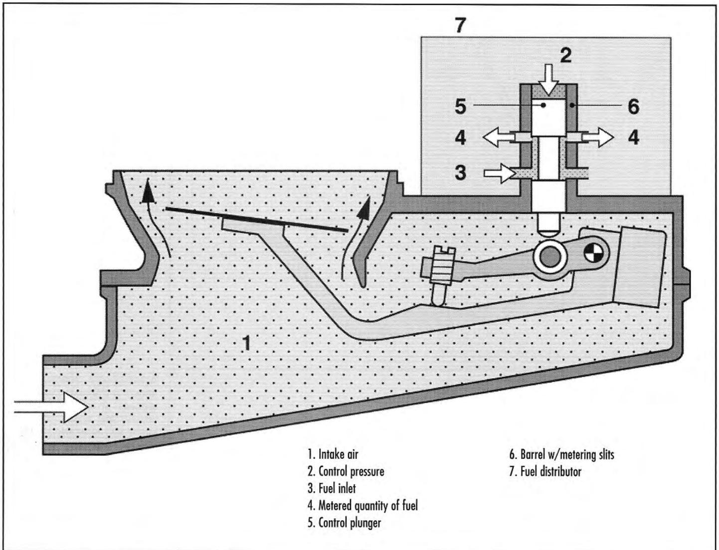
Within the air meter, the sensor plate pushes upward on the control plunger through an intermediate lever. Plunger movement is always upward for more fuel, so on downdraft sensors the pivots of the intermediate lever are reversed. (Robert Bosch Corporation)
