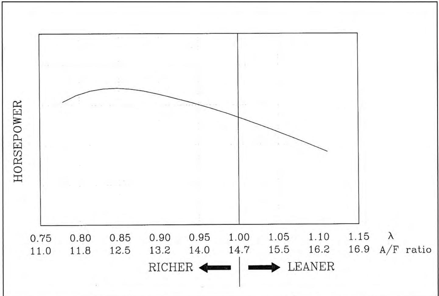
Maximum power is produced with a mixture just a bit richer than the chemically "correct" ratio. Power tapers off sharply with increasing richness beyond that point, and more slowly as the mixture is leaned-out.
