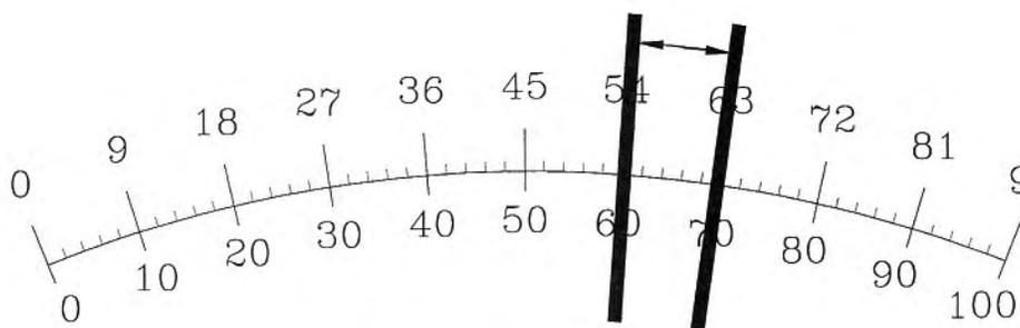
A reading around 60–70 degrees (about 55–65% duty cycle) means the lambda valve is trying to drop the control pressure to richen up an excessively lean mixture.
