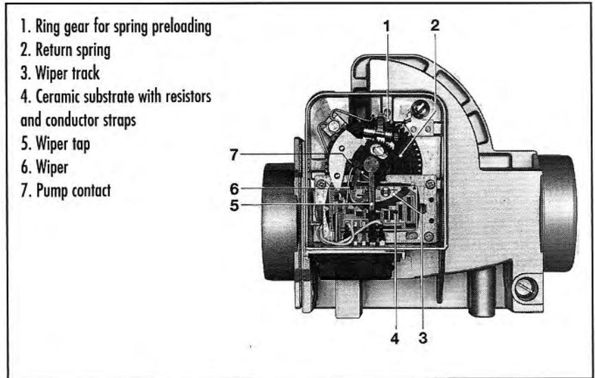
**The vane-type air meter of an L-Jetronic system, viewed from the electrical connection side. (Robert Bosch Corporation)**
