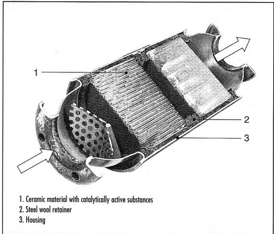
**Construction of a three-way catalytic convertor. Convertors are essential to meet current emissions limits, but can only do their job if the air/fuel mixture fed to the engine is held very close to the chemically correct ratio. And to achieve that, a lambda (oxygen) sensor is essential. (Robert Bosch Corporation).**
