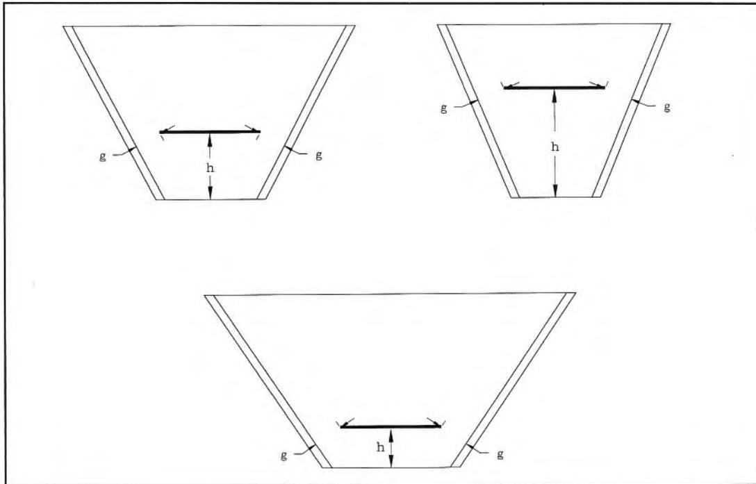
The height (h) of sensor plate lift needed to obtain a certain flow area (g) depends on the rate of taper of the funnel.
