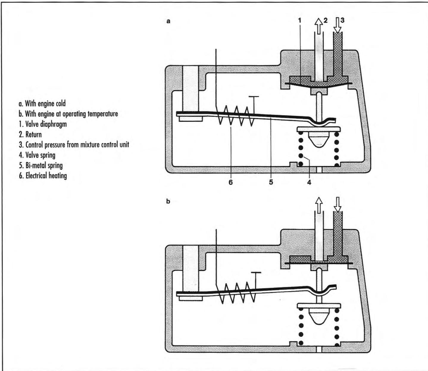
The control pressure regulator, previously termed the "warm-up" regulator (a) with the engine cold (b) with the engine warm. (Robert Bosch Corporation)
