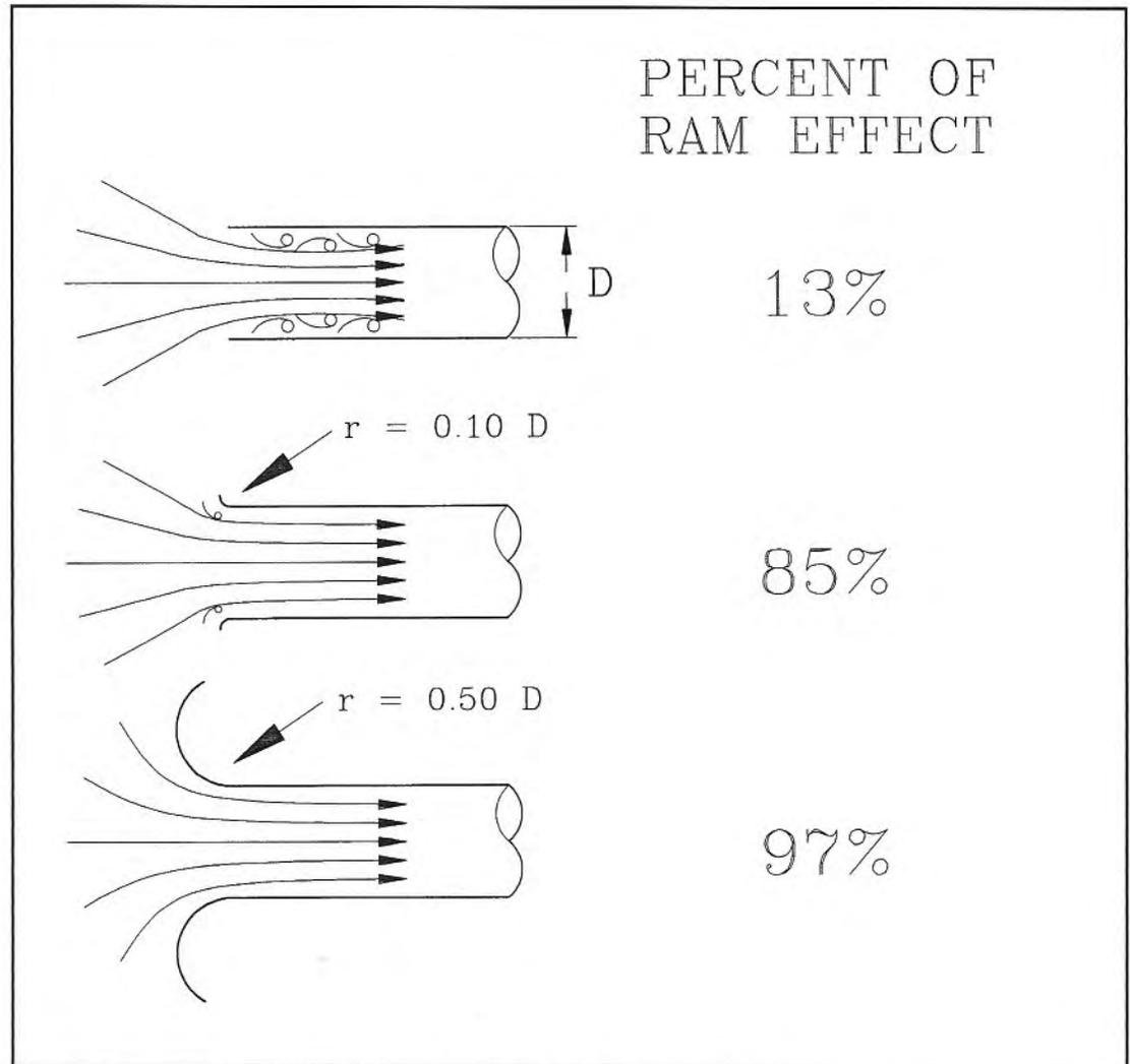
Most of the benefit of tuned "ram" pipes is lost if the entry to the pipe is sharp edged. A smoothly radiused edge is necessary to get maximum benefit; a large radius is better than a tight one.
