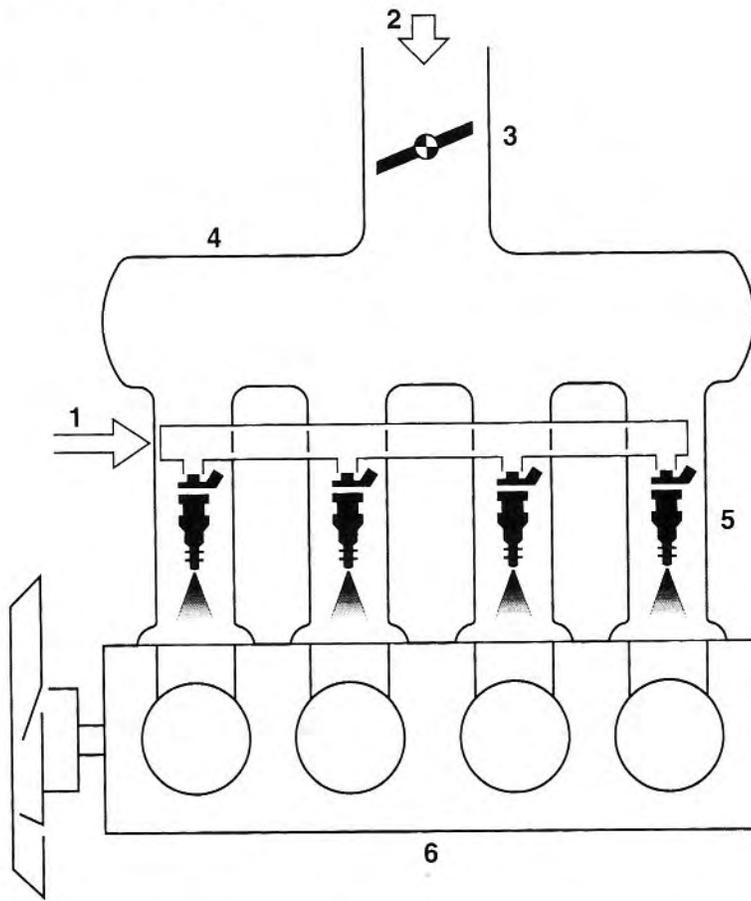
**Multi-point injection ensures equal mixture strength at each cylinder. (Robert Bosch Corporation)**
