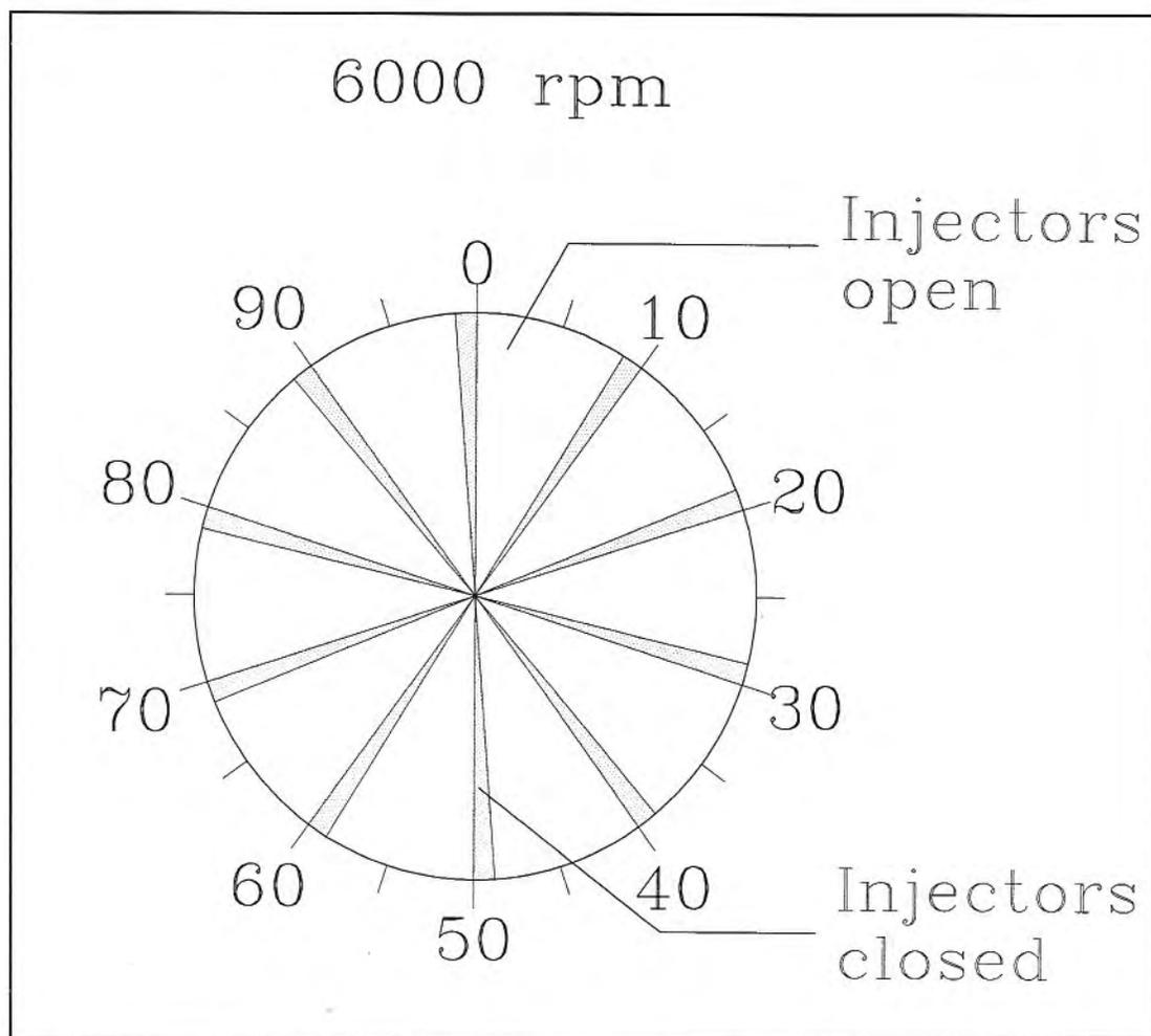
At a given supply pressure, the upper limit to rate of fuel delivery may be set by the injectors—even though they spend almost all the time "on," they can only just keep up with the demands of an engine making maximum power. Bosch recommends that their duty cycle should not exceed 85% or so.
