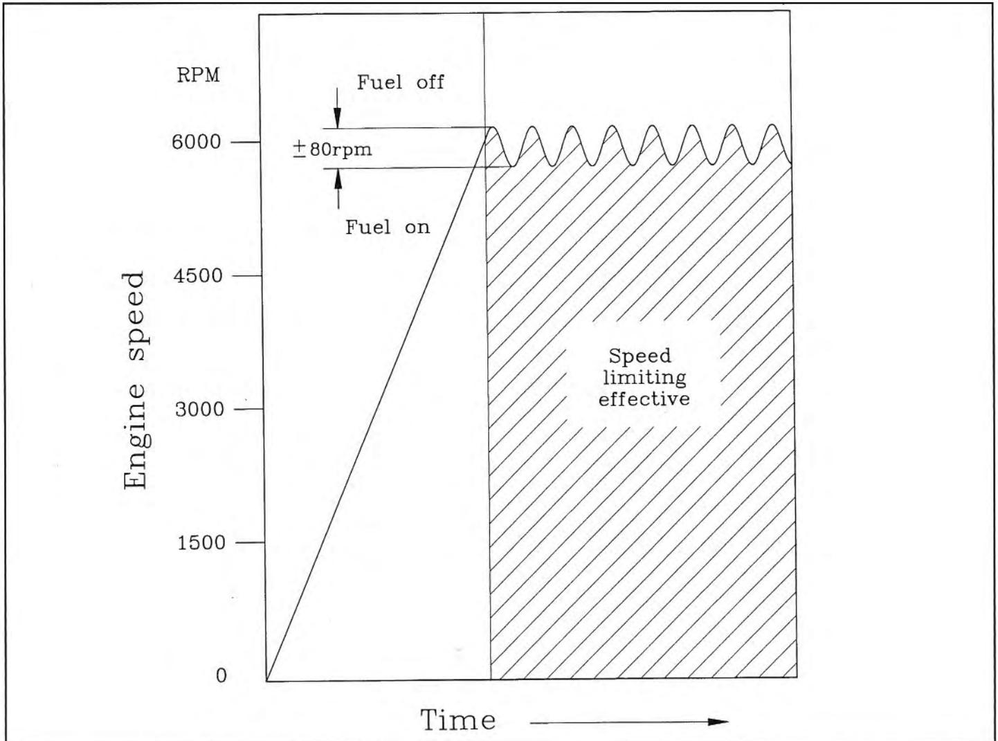
Another feature of Motronic systems is a built-in rev limiter. Although engine rev limiting can be achieved by interrupting the ignition, this can cause rough running and backfires and be hard on the machinery. Cutting off fuel is smoother, and reduces emissions, too. Once the preset rpm limit is reached, the cut-off rapidly oscillates between "fuel on" and "fuel off," with about  $\pm 80$  rpm between the two states.
